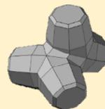
Realizing high stability against waves and flow by strongly interlocked 4 legs. For places with high waves, it is an economical wave-dissipating block that does not use reinforcing steels inside.
