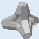
A radiation-type wave dissipating block with 4 hollows on the surface. Interlocking of legs and hollows prevents damage from spreading and improves stability against wave force and wave dissipating effect.
